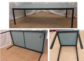
Note 1: This item was tested to sizemark 4/5/6 Normal for strength, durability and stability. Dimensionally the sizemark is between 5 and 6 (indicative only). The table/desk work height is 725 mm.
